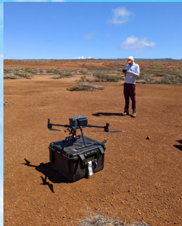
Timo Sullivan of Island Conversation preparing the Matrice 300 drone with a H20T thermal sensor to take flight
